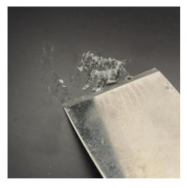
If there has some glue hard to be clean off by scraper, please put the plate back and set the bed temperature to be 230℃ and wait for about 30 minutes. Then try with scraper again.
