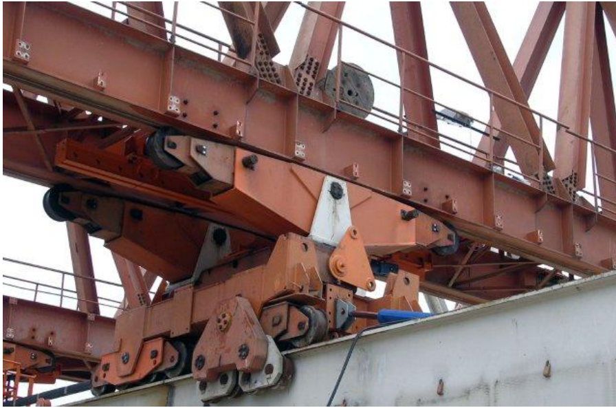
Figure 7: 32-roll saddle for 635ton service load
