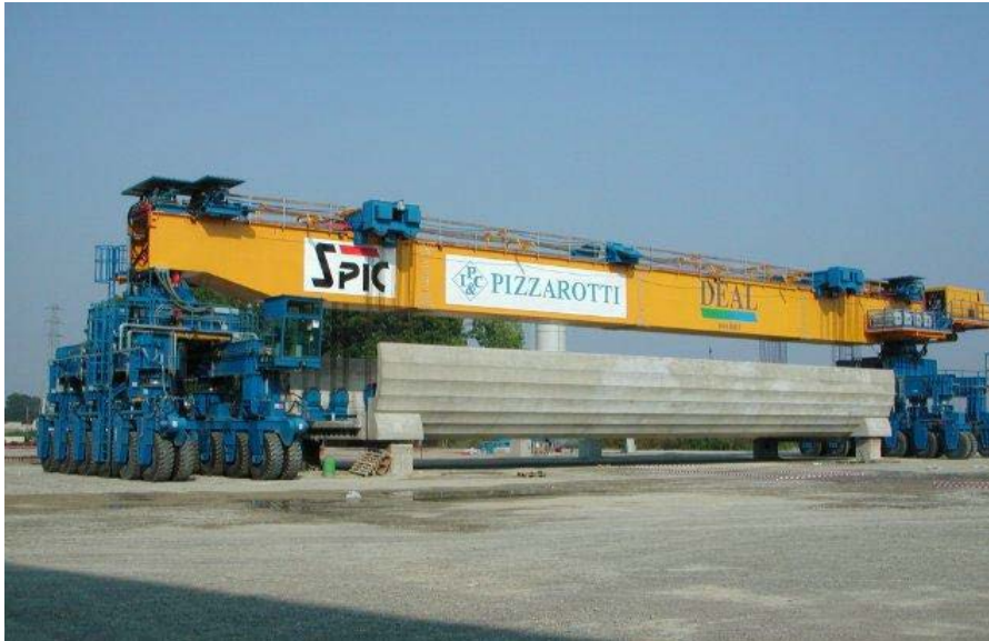
Figure 34: 58m, 321ton carrier for placement of 31.5m, 740ton single-track HSR spans
