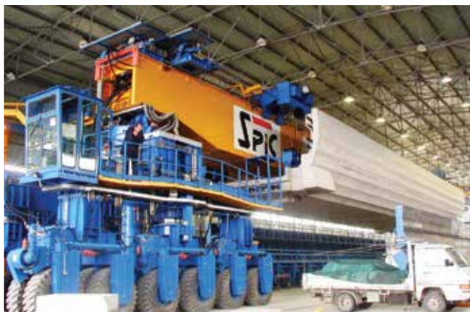
Figure 8. Beam transfer to the storage platform with a portal carrier with pivoted tractors.
