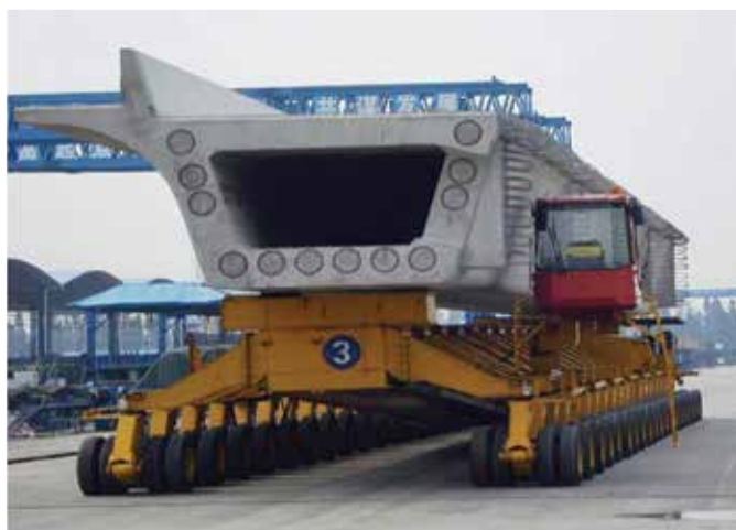
Figure 9. Extraction saddle of a tire trolley for 4000 kN (900 kip) single-track box girders. Courtesy of BWM.
