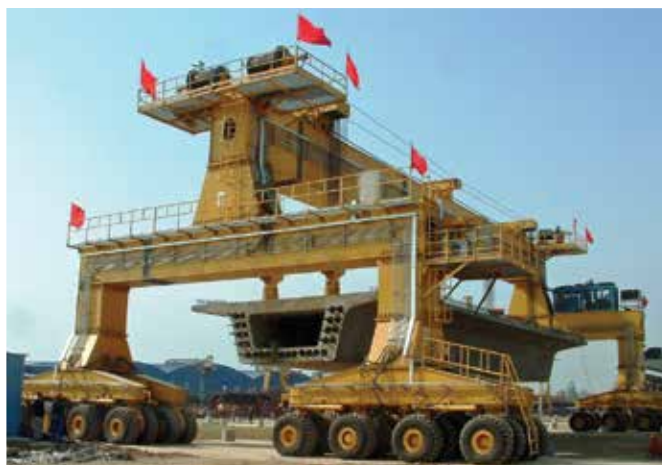
Figure 7. A 9000 kN (2020 kip) dual-track box girder handled with a 64-wheel portal crane. Courtesy of BWM.
