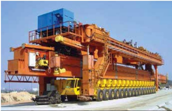
Figure 13. Main frame and two-span underbridge repositioned with the tire trolley. Courtesy of BWM.
