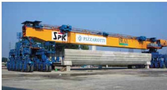
Figure 14. A 58 m (190 ft), 3200 kN (720 kip) portal carrier with pivoted tractors for placement of 31.5 m (103 ft), 7400 kN (1660 kip) single-track U beams.
