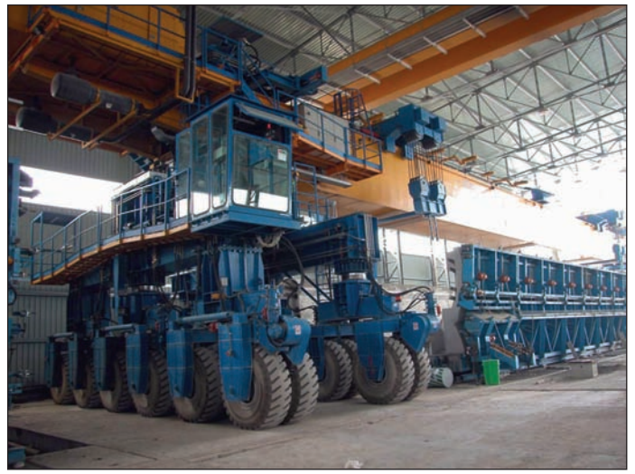
Fig. 4: Span lifting from casting cell
