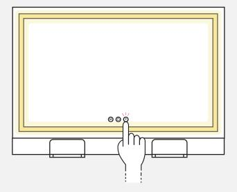
3 / Tap mode (M) button to cycle through 3 light setting options (Neutral White - Natural Daylight - Soft White).
