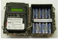
**TIP:** It's good practice to make sure the gasket is seated properly and no debris has gotten into the gasket area each time you open and close your camera. It is also a good idea to check that the windows on the front of your camera are clean.
