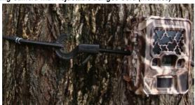
We recommend that you mount your camera about chest height and angle it slightly downward. This is optimal for detecting animals in the field of view of the camera as well as for accessing the camera's card, batteries, and controls.
