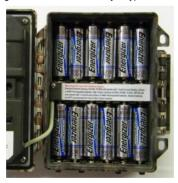
**Warning!** Do not mix battery types! Damage to the camera can result and your warranty will be voided if you mix battery types.
