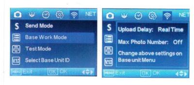
**Upload Delay Settings:** Default setting is 30 mins. The base unit will wake up and communicate with LC32 cameras every 30 minutes. If there are 3 linked cameras (S1, S2, S3) connected, the base unit will wake up and check on S1. If there are new
