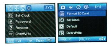
**SETTING THE CLOCK:** Press the ▼ button one time to highlight the **Set Clock** option. Press **OK.** You will see the following screen.
