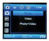
Under the Camera Mode tab, select whether you want Photo, Video or Picture+Video. Press **OK** to save. Press **MENU** to go back to the Camera Mode and **Customize** screen. Press the ▼ button one time until **Customize** is highlighted in blue. Press **OK**. If you chose Photo or Picture+Video Video Size
