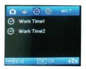
If you only want your camera to be on during part of the day each day you can set the **Work Time** function(s). Press the ▼ button to highlight the **Work Time 1** option. The default setting is **OFF**. Press the ▲ button to toggle the setting to **ON** and press **OK**.
