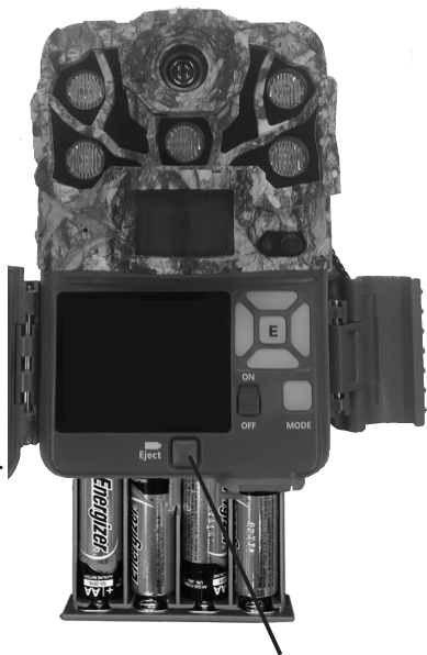
Battery Eject Button
