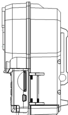
No force should be required to insert the card, should it feel as though the card will not freely slide into the slot, remove the card and check for any obstructions.
