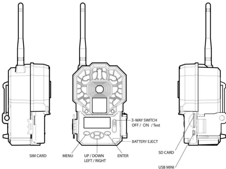
**(NOTE: You'll need to screw the supplied antenna into the top of the camera.)**
