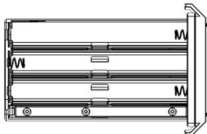
New, Alkaline or Lithium, 'AA' batteries must be inserted with the orientation as shown on the tray. As with most electronic devices the negative ( - ) orientation of the batteries should be against the springs. Failure to insert the batteries properly will cause damage to the unit. Remember camera uses (12)'AA' batteries, six on each side.
