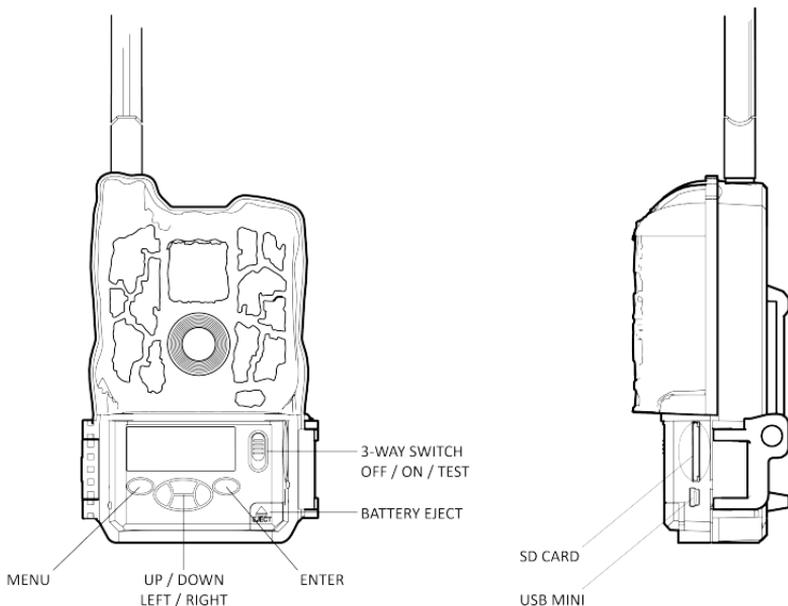
**(NOTE: You'll need to screw the supplied antenna into the top of the camera.)**
