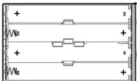
New, Alkaline or Lithium, 'AA' batteries must be inserted with the orientation as shown on the tray. As with most electronic devices the negative ( - ) orientation of the batteries should be against the springs. Failure to insert the batteries properly will cause damage to the unit. Remember camera uses (12)'AA' batteries, six on each side.
