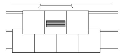
**Step 4: Protect the opening in the felt.** As close to the vent as possible, a folded piece of roofing felt needs to be inserted into the felt to act as a weir to divert any rain water driven onto the felt, around the aperture.
