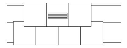
Step 3: Position and secure the vent. Continue tiling .
