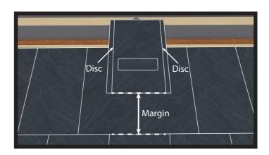
**Step 7:** Place the vent in position and secure, ensuring the tail of the vent is at the correct margin. If required insert complete copper disc rivets to slots.
