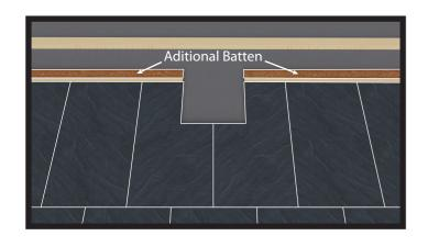
**Step 5:** To secure the ends of the cut batten, nail further batten above the cut batten and tosh nail the ends. (Recommended to span two rafters)
