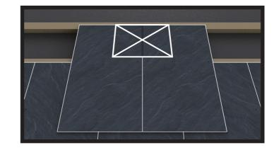
**Step 3:** A vertical cut needs to be made from the head of the slate to where the slate meets the batten. Remove slate and trim.
