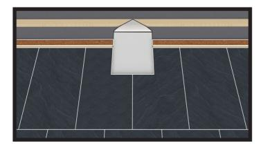
**Step 6:** Carefully cut away the felt to the area of the removed slate. Cut the top section diagonally and pin back to the batten above.
