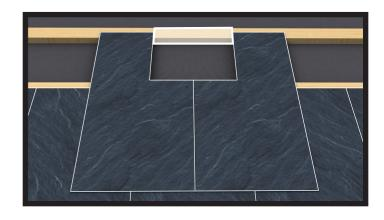
**Step 4:** Re-position slates and fix securely. Carefully cut batten from between the removed section of slate.
