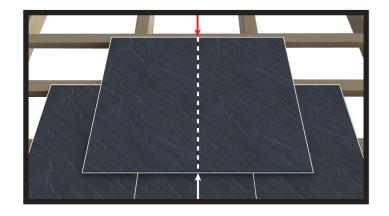
**Step 1:** Two slates will need to be trimmed. **Ensure the perp formed by the two slates falls between rafters.**
