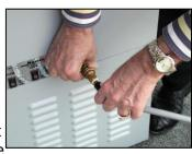
to unit. Note: These two connectors must be all the way in for solution pump to run
