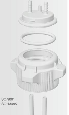
Foxx Life Sciences' **Versa**Cap® Filling and Venting closures are aseptic handling solutions for pharmaceutical, biotechnology, and laboratory liquid transfer applications. All closures can be used on bottles and carboys with 53B, 83B, or 120mm closures. The pre-mounted lengths of platinum-cured silicone tubing allow for easy customization of carboys and bottles.
