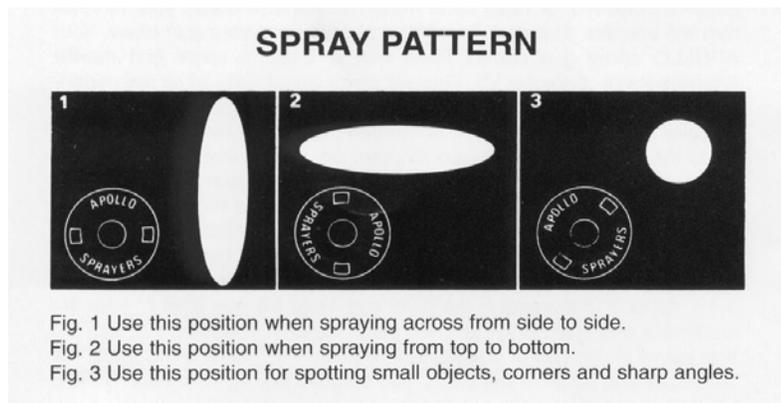
Your Mist Applicator offers you many options. You can adjust (click) the air cap (#2) to three positions. One will produce a horizontal pattern for spraying across, another will produce a vertical pattern for spraying up and down, and the third will produce a round pattern.
