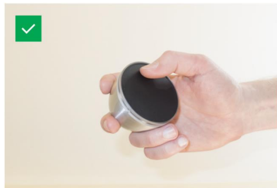
Hold it at an angle to register the top of the touchpad
