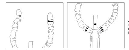
• Check the condition of the safety stitching (above/below) Look for any threads that are loose, worn, or cut.
