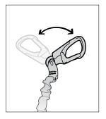
• Move the connectors to inspect the hidden parts
