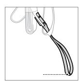
• Look for wear and damage due to use, especially at the girth hitch (cuts, fuzziness, chemical residues...)
