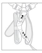
• Check the condition of the safety stitching (above/ below) Look for any threads that are loose, worn, or cut.
