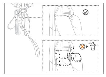
Then, check whether the energy absorber has been subjected to shock-loading (verify that the energy-absorbing webbing isn't torn).
