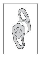
• Check the condition of the side plates (marks, deformation, cracks, corrosion, wear...).
