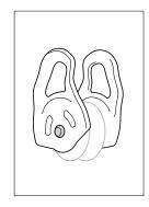
• Check the condition of the rivets (marks, deformation, cracks, corrosion, absence of play...).
