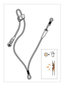
• Look for wear and damage on the sheath due to use (cuts, fuzziness, chemical residues...)
