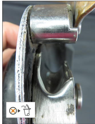
• Cam groove worn to wear indicator
