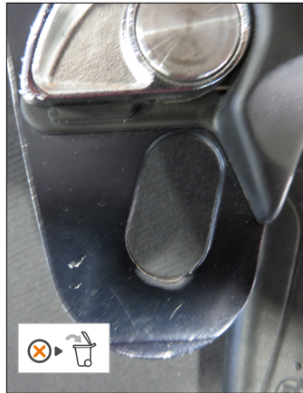
• Attachment hole deformed by a shock load
