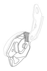
• Check the condition of the friction plate (marks, deformation, fouling, cracks...).
