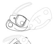
Check the condition of the rivets (marks, deformation, cracks, corrosion, absence of play...).
