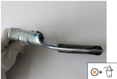
• Damaged attachment holes
