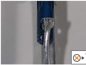
• Bad gate/nose alignment
