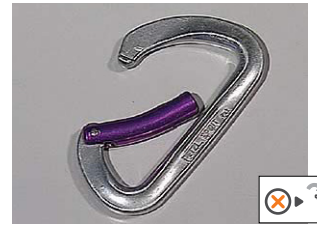
• Defective return spring
