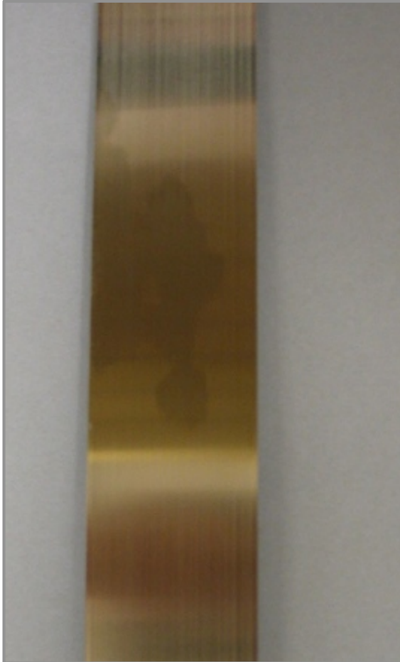
Figure 9. New spring showing absence of any defects visible to naked eye.
