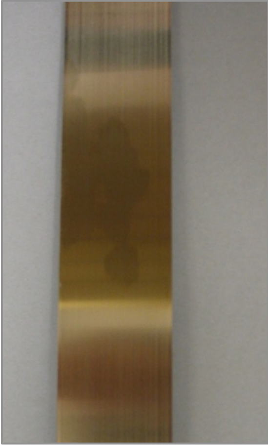
Figure 6. New spring showing absence of any defects visible to naked eye.
