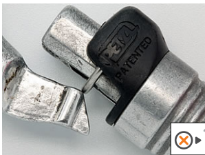
• Defective locking system
