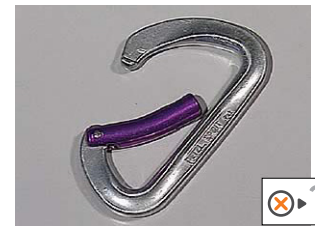
• Defective return spring
