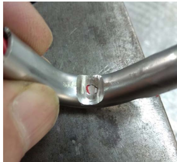
Figure 23: Worn abrasion guard - needs replacement
