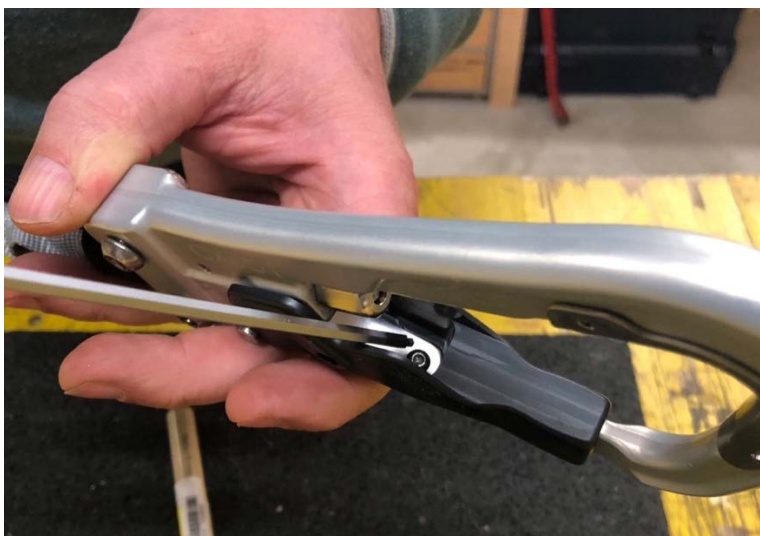
Figure 21: Fastening and gluing the screw
