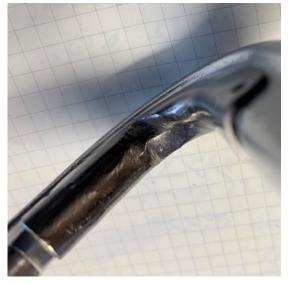
Figure 21: Slightly worn abrasion guard - does not require replacement
