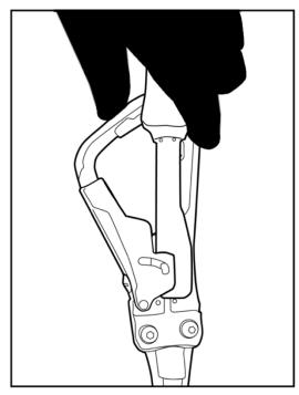
Figure 29: Use of the Carabiner Removing Tool with safety gloves
