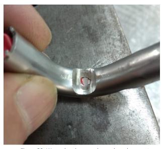
Figure 22: Worn abrasion guard - needs replacement
