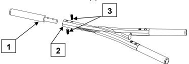
Cut the wire ropes so as to have clean cuts and insert the wire ropes into the ferrules all the way to the end (allow for some slack in the wire ropes) Swage the tubes as per the indicated order (from 1 to 6 as per the diagram below).
