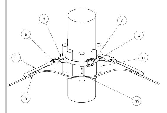
Place the protection logs (a) so as to avoid any contact between the metal band (b) and the tree.
