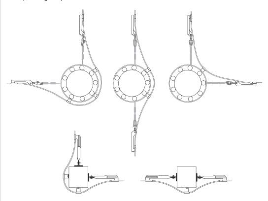
In some cases the metal brackets (m) will be fixed on bracket inverters (g) depending on which way the lifeline is installed around the support.
