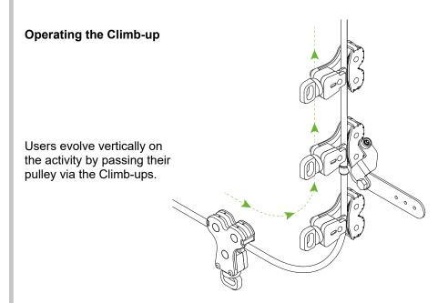
With a 0.6m/1.96' lanyard and the Climb-ups installed 0.6m/1.96' apart, the highest fall factor is 3. Tests have been carried out with a maximum weight of 140 kg /308 lbs /22 stones and a minimum weight of 30kg /66 lbs /4.72 stones so as to ensure that the maximum deceleration is inferior to 6G.
