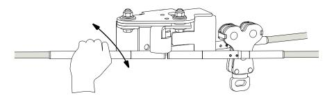
The instructor can condemn the crossing or oblige users to use a chosen crossing by blocking the mobile part with the pin (7). A bolt can replace the pin.
