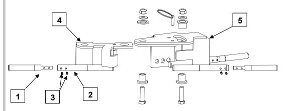
**2 -** Fit the body onto the support with screws, bolts or champ plates. Use the holes (6) to do so.
