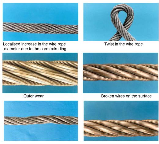
Localised reduction in the wire rope diameter (hollow strands)
