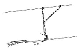
**3** – Fit the chain onto the upper wire rope with 2 wire rope clips. Connect the chain and the energy absorber to the brake with 2 stainless steel  $\emptyset$ 7mm Maillons rapide. The brake must be 0.5m /1.64ft from the extremity of the zip line arm.
