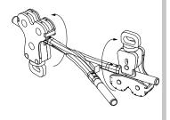
2- The user chooses to go the other way and therefore has to tilt the pulley so that it is upside down, then passes the pulley into the swapper and tilts it back the right way up once he/she is on the right path (see the diagram opposite)
