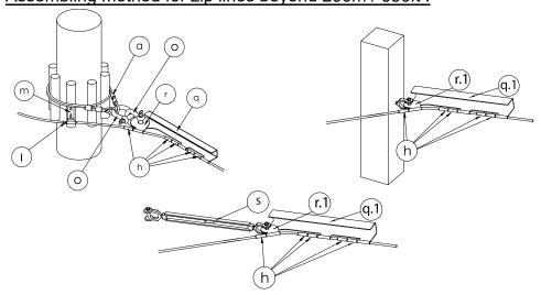
To increase the life-span of zip line wire rope, we recommend using swaged galvanized steel wire rope - 6x26, metallic core, which can be joined to the lifeline with connecting ferrules. (refer to chapter 3.13).
