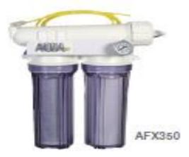
Dolphin R/O systems have a highefficiency 1-micron sediment prefilter, 2-micron carbon block prefilter and a high-flow/high-rejection Dow<sup>®</sup> R/O membrane providing excellent water purification. The 160-psi pressure gauge and clear 10" filter cartridge housings allow full system monitoring. Quick disconnect fittings, filter wrench and hose bib attachment are included.
