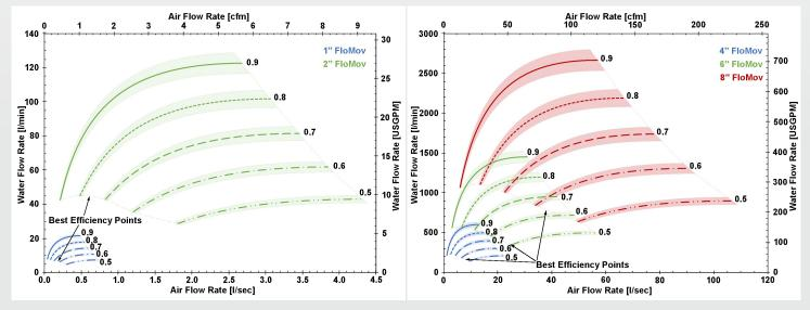
FloMov pump performance curves for submergence ratios from 0.5 to 0.9. Shaded areas on the curves represent the expected variability in pump performance due to several factors including variations in installation, different inlet/outlet fittings, varying air inlet flow distribution and varying aeration needs.
