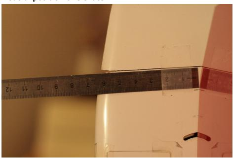
**Control surface settings:** All dimensions are measured at the root of the control surface and at the trailing edge.
