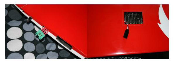
Before installing the servos, put in neutral for the aileron servos. Provide an offset of 20  $^{\circ}$  for the flap servos. This is to be a large movement of the flaps.
