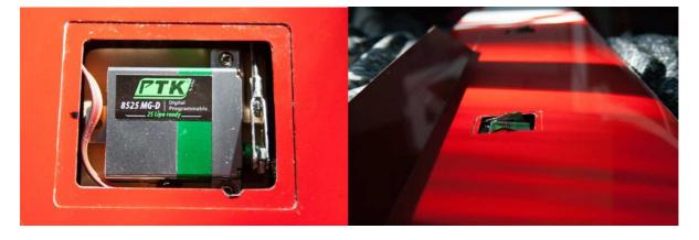
To lock the rod or the operating clearance is too high, you can add a drop of cyano on the spreader and the horn.
