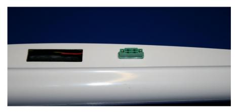
The servos plate does not receive servos here but contributes to the strength of the fuselage. It is therefore necessary to paste.
