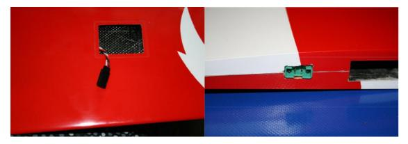
Before installing the servos, put in neutral for the aileron servo. You can now install the servos and connect the rods. Favor a mechanical adjustment.
