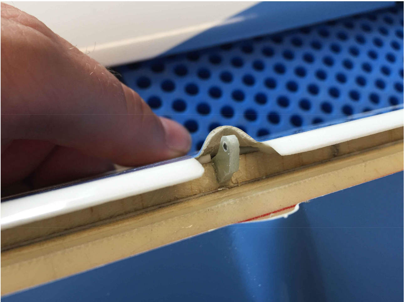
control horn fixed with thin CA. after that glue it in save with thickened slow cure epoxy
