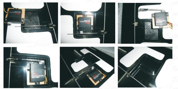
• Make up control rods and clevises using the parts supplied.
