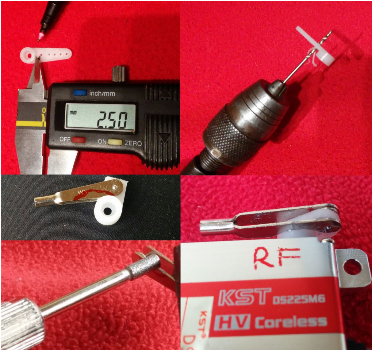
Figure 6. Prepare the servo horns and clevises for the wing servos. First drill a hole through the servo horns (for choice of drill see figure 4) 2,5mm outside the servo horn base (upper panels). The clevises will need to be milled on the bottom side to allow for full movement respective to the servo horn shaft (middle panel and lower left panel). Once that is done the clevis allows for full movement when mounted on the servo horn (lower right).
