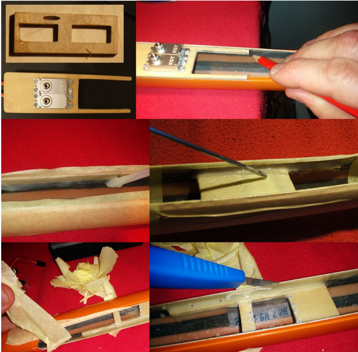
Figure 16. The servo board: To save precious space in the fuselage cut out your own servo board from 4 mm plywood using the supplied one as rough template (upper left). I used 3mm plywood and laminated one layer of 80g glass on top and bottom. Make sure the board fits perfectly but tightly in the fuselage at your desired position. The servos should be mounted in the board when you test fit it in the fuselage. Thereby, you can estimate how deep in the fuselage you may mount it. Mark servo board positioning in fuselage (upper right). Cover outside of fuselage with masking tape to protect from epoxy. Now mix UHU Endfest epoxy and smear a thick layer into the fuselage where the board should sit (middle left). The servo board itself is also covered by masking tape. Just leave about half a cm blank on the sides for good attachment to fuselage by the epoxy. Smear epoxy on bottom and top of the sides of the board and press it into marked position in the fuselage (middle right). After about 4-6h of curing at room temperature, when the epoxy has hardened but isn't yet bullet proof, remove masking tape and if there are any unwanted epoxy residues cut off with stanley knife (see lower images).
