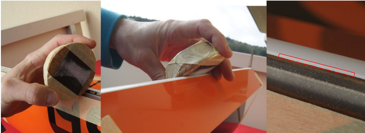
Figure 2. Taper the control surface sealing lips: First cover your working table with a soft cloth, such as a fleece blanket to protect the wing surfaces. Next, apply masking tape onto the respective wing and control surface (left panel). Now, use a sanding block to bevel the sealing lips carefully. Be careful to keep the “angle of attack” constant over the whole length of the sealing lip, as seen in the middle panel. This will help to generate a pointed leading edge (see right panel, red box) that won’t catch the wing surface, even after coming back in from maximum deflection.
