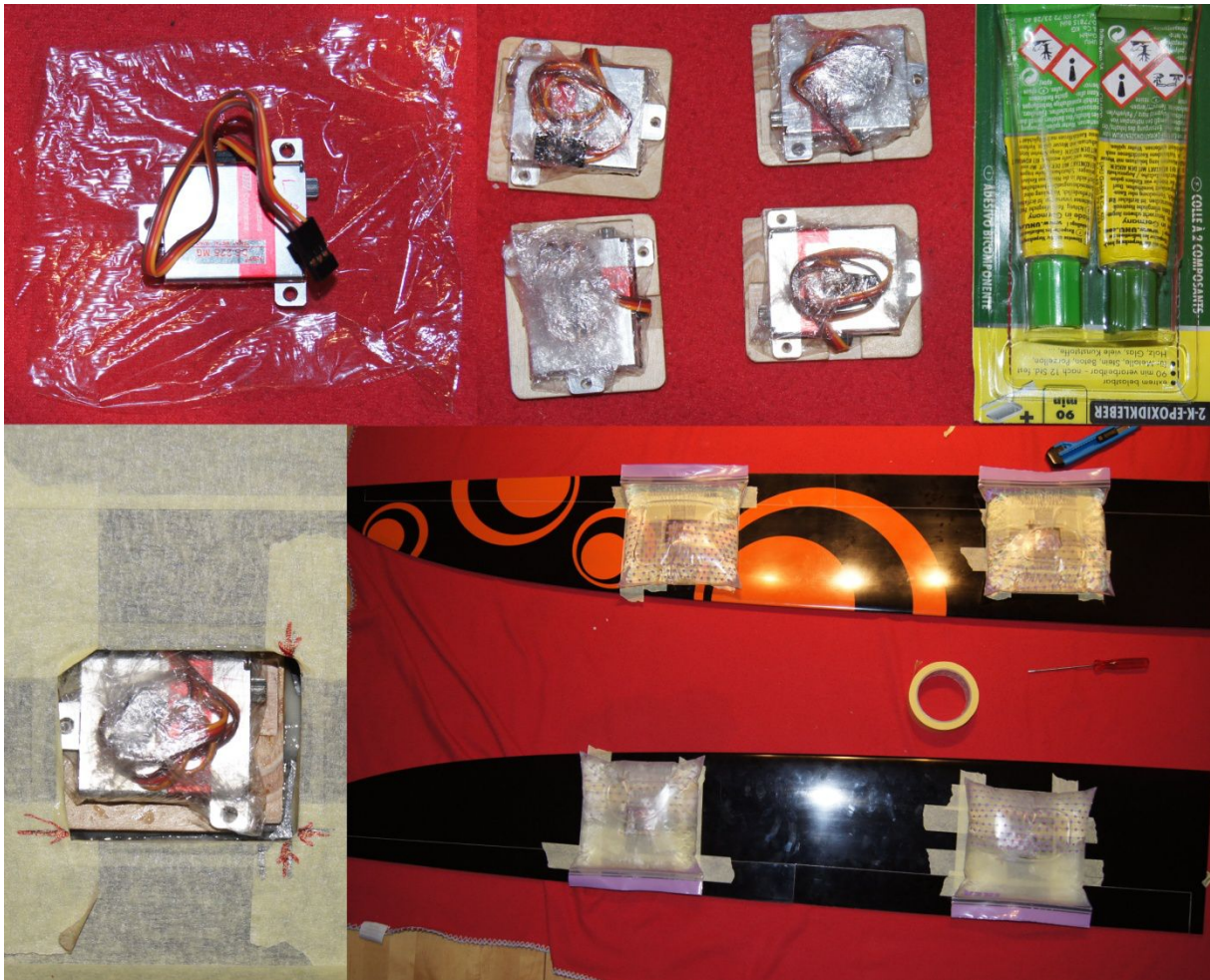
Figure 8. Fix the servo frames in the wings: First, wrap each servo with saran wrap (upper left). Next, briefly sand servo bays and bottom of servo frames and push each (saran wrapped) servo into its respective servo frame (upper right). Now mix the endfest epoxy, add some cotton flakes (or microballoons) for thixotrophing it and smear it into the fine sanded servo bays and onto the bottom of the servo frames. Bring the frames with the servos into the marked position in the wings (lower left). A nice trick for tight attachment of the frames is to put water filled plastic bags on top of them (lower right). This ensures even weight distribution and is simple. Putting metal weights on top of servos however, is good too.
