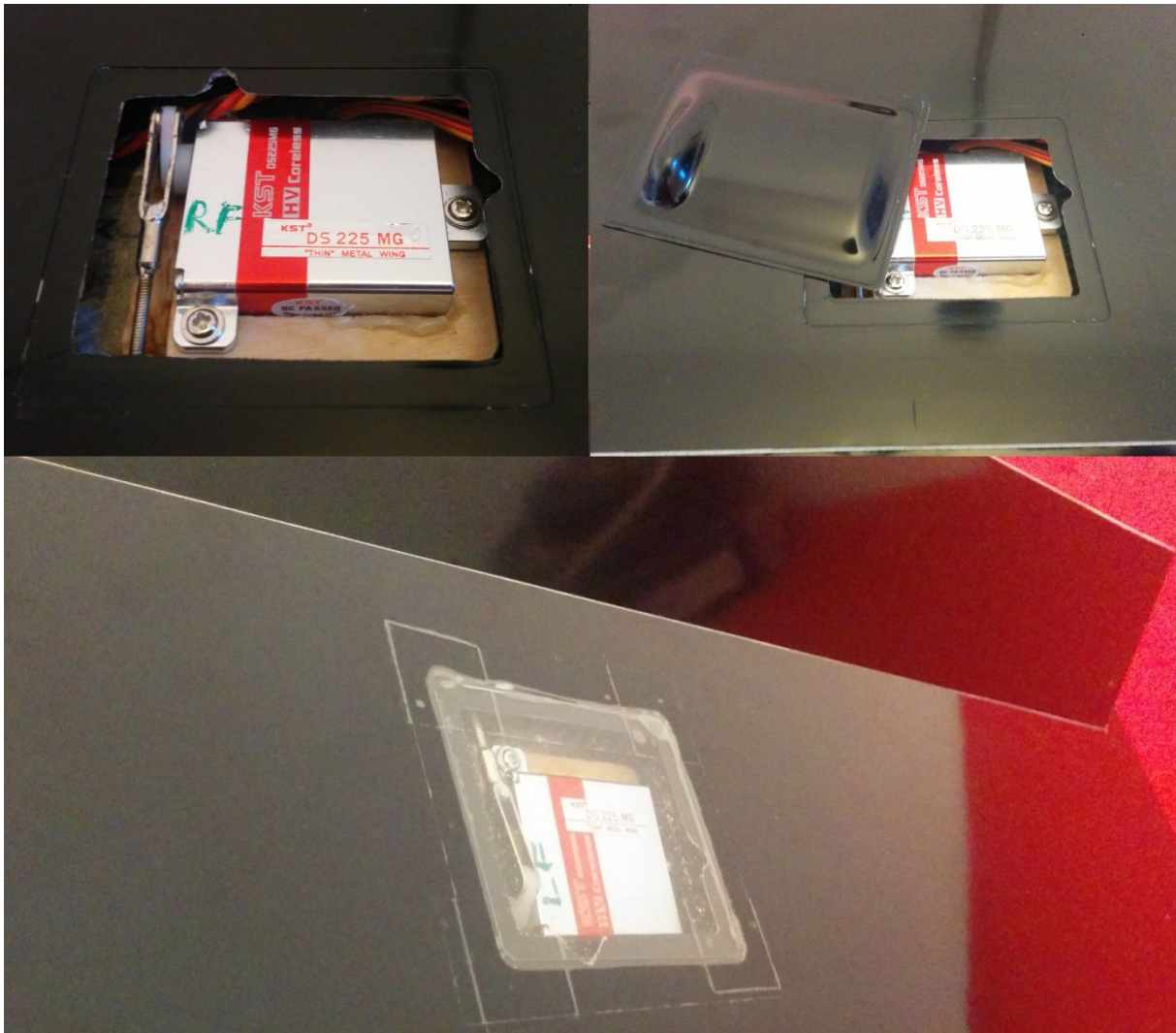
Figure 12. Mount the wing servo , in their respective servo bays, in the readily prepared servo frames (upper left). Servo arms should still be in the right positions as prepared under figure 9, above. Therefore, you can also easily attach the linkage system at the servo horns and at the control horns. Again, one of the two clevises on each pushrod has a grinded side, which needs to face the servo horn base, to allow for full movement. Once each servo is properly installed and connected (upper right), the supplied servo covers will fit easily on top of them (upper right). However, for better aerodynamics you can substitute them for plain plastic plates that were cut to size, accordingly. Fix them with transparent tape, as usual. No structural support is provided or needed by any of those servo covers. I personally used transparent plastic plates so that you can see the servo below (lower image).
