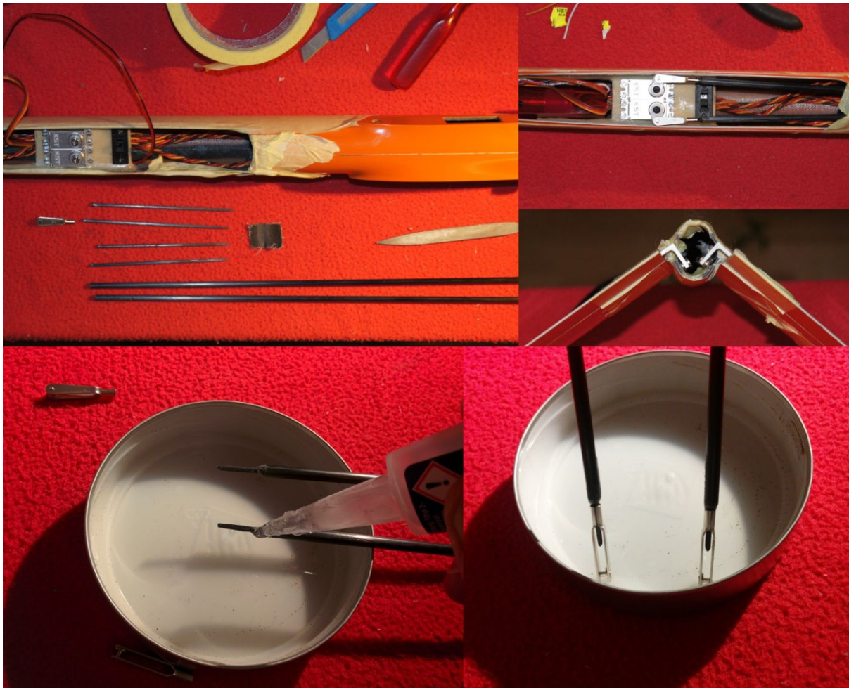
Figure 17. V-Tail linkage: Upper left. Use the long carbon rods that are delivered with the kit (figure 1g). Fiddle them into the fuselage. Servo horns need to be in 90° position to servos and V-tail control surfaces in strak. Now mark each rod 4 cm in front of the respective V-tail linkage horn and 4cm behind the servo horn. Take them out of the fuselage and cut at marks. Instead of the supplied threaded rods (figure 1b), I suggest to use 1,5 mm carbon rods for the connection of the clevises. Cut the 1,5mm rods to four 10cm pieces (upper left) and laminate those 7-8 cm deep into both sides of the thick carbon rods using UHU endfest. Let cure over night. In the meanwhile, trim the clevises as seen for wing servo clevises in figure 6. Once epoxy has cured, the clevises can be screwed onto the rods with force. To make it easier, you can grind off some material from the end of the rods using glass paper. Now, adjust clevis positions so that the V-tail control surfaces are perfectly in strak when the servos are in 90° positions (upper right). Permanently attach clevises using cyanacrylacetate super glue (lower images). As soon as hardened you can mount the ready made pushrods in the fuselage and you will be happy that there is close to zero tolerance on the V-tail.
