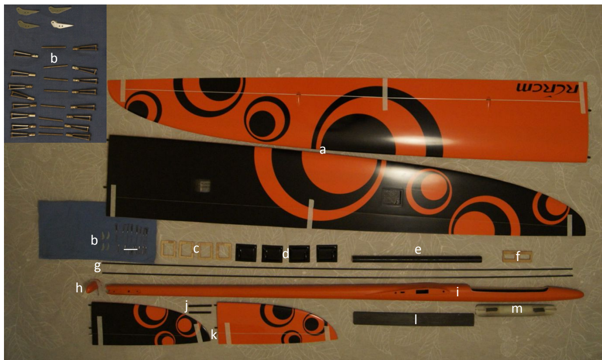
Figure 1. List of Strega kit parts: (a)Wings; (b)accessories [see insert on the upper left; 16 clevises, 8 threaded rods, 4 control horns]; (c)wing servo mounts; (d)wing servo-bay covers; (e)ballast tube; (f)fuselage servo tray; (g)carbon push-rods; (h)tail piece; (i)fuselage; (j)V-tail joiners; (k)two piece V-tail; (l)wing joiner; (m)canopy.
