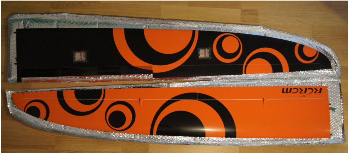
Figure 13. Readily assembled Strega wings. Test for proper function of the wing RC system as soon as the fuselage sided wing servo plugs and corresponding receiver cables are installed.
