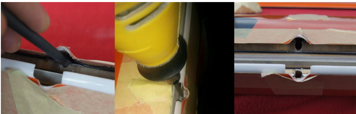
Figure 3. Drill holes for control horn installation: You can use a round file to file a whole into the wing back shear web exactly below the pushrod exit hoods (left panel). Alternatively, you can also use a small electric drill with a rotary bit (middle panel). In this case however, be careful not to break through the wingskin. If you place one finger underneath it you will feel the vibrations once you get critically close to the surface. The flap and ail shear webs have to be treated the same way. In the end they should all look like in the right panel.
