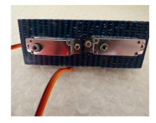
Before final gluing, I mount the tailplane units with the controls we previously prepared. Then place the support plate in the fuselage, cut the pushrods to the appropriate length. Be careful with the height of the horns, they should be adjusted to prevent friction against the fuselage:
