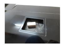
To prepare the bonding, it is important to protect servos with wax. We polish with this wax the surfaces which may be in contact with the glue. This will allow to remove the servo if necessary later.
