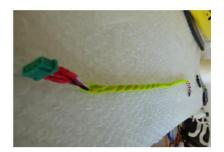
The green sockets should fit well on the fuselage, however it is possible that it could be necessary to adjust with a file. The operation is simple to perform.
