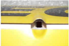
Before continuing, it is important to do a test without glue Ensure that the pushrod move freely without touching the beam.
