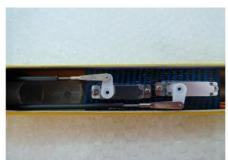
We can then paste the support with Epoxy + glass bubbles. A preliminary polishing will get a better bonding.
