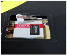
The flaperons are treated differently: the flap is still in neutral position but the servo arm is tilted by 30 ° to the spar. This will allow to obtain the necessary travel down.
