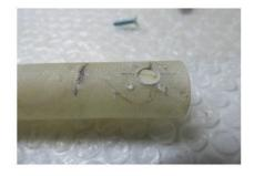
To let the pieces of ballast enter, cut the tube in half (see photo). We then stick the Tiger nut on the tube.
