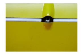
You should adjust pushrod to the correct length and check that everything is in line before installing the servo support. A glueless installation is required to ensure correct location. In the assembly, we used 10 mm servos. (Kst 125mg)
