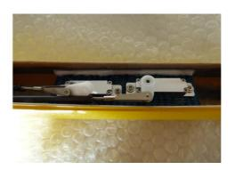
Supplied RCRCM wiring is adjusted to the correct length. The fuselage being very narrow, I preferred to use a sheath to join each wiring harness.
