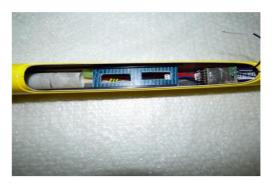
The ballast hold delivered by Rcrcm is a simple tube made of fiberglass. We will need a Tiger nut with the necessary screw. First, we find the good location of the Tiger nut. It is necessary to drill the four holes.
