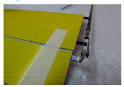
A significant element in the fuselage: the ballast hold. This takes a lot of space in the fuselage and we must foresee now its integration. This hold will allow you to change the wing loading depending on weather conditions.
