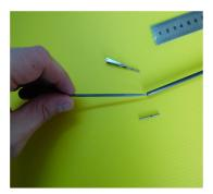
The next step is to paste the pushrods with clevises. It is necessary to respect the same length for each one. Use 30 minutes Epoxy glue.
