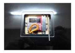
*To paste the support, it is important to polish the inside of the wing for better bonding with carbon.*
