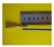
It is important to prepare bonding. It is necessary to file the inside of the tube to get a better grip for the Epoxy glue. The operation is to be done for both controls.
