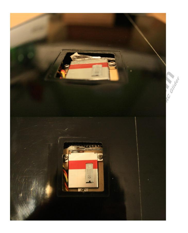
You can now set up the servos cover. The cover is here glued to double-sided tape
