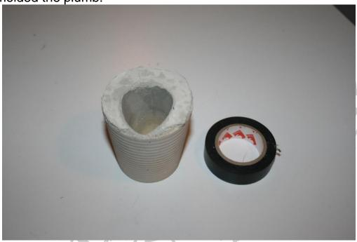
Take a latex glove, place it on the SPLIT nose. Fill a plastic cup with plaster and dip the Typhoon + nose. Once dry, remove the fuselage.
