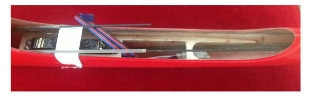
Once cured, intall the servos tops (with coupler / clevis attached), centralise the elevator and rudder servos, and cut the pushrods to the required length (a fine toothed razor saw is ideal for this operation). Upon completion, roughen the pushrod inners with high grit (smooth) glass paper and glue the couplers to the pushrods using 30 minute epoxy.
