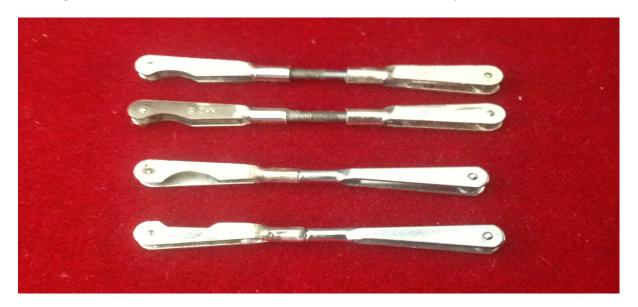
With the radio switched on (and servos centralised), connect the pushrod to the control surface horn and servo top, and rehearse the process for applying epoxy to the servo mount. Once satisfied with
