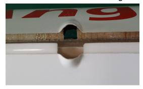
Glue the horn, make sure the horn will not touch to the wing skin, connect the horn with clevis.
