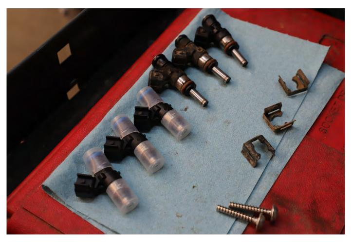
• PLEASE BE SURE TO HAVE PROPER SAFTY EQUIPMENT AS THE <u>FUEL RAIL</u> <u>May be presserized.</u> And by removing an injector, it will release that fuel. Please be aware.
