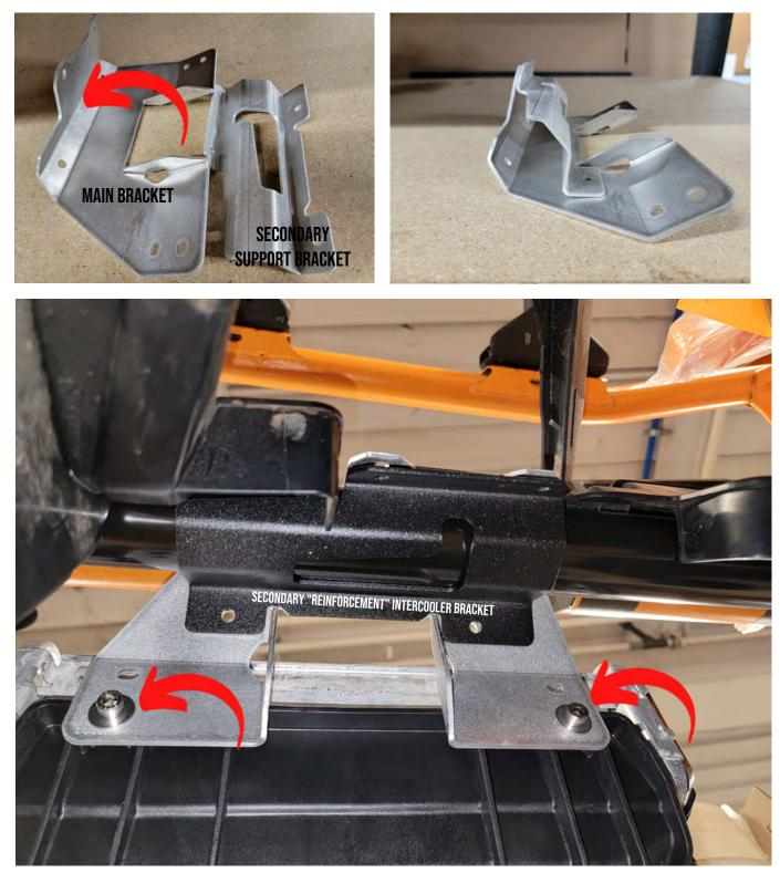
• <u>TECH TIP UPDATE</u> • THE REINFORCEMENT BRACKET WILL HAVE RIVET NUTS INSTALLED TO EASE INSTALLATION.
