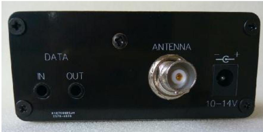
Power connection: Any DC power 10-14V, 1A connect to power jack.
