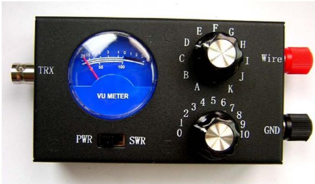
The band switch S2 counterclockwise in the end, making the mark target exactly to A. Switch dual capacitor C5 counterclockwise in the end, making the mark target to 0, tighten the knob, and the installation is over.
