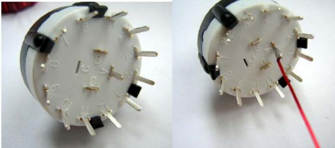
The 1-12 feet of band switch S2 should be bended outward, in that case magnet ring L1 can be put within .Solder foot A with the 30mm 24 # enameled insulated wire.
