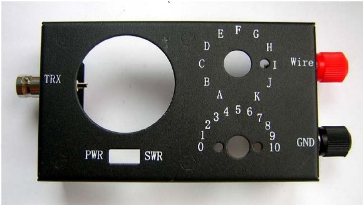
Install the BNC seat and two binding posts in the corresponding position on the cabinet..
