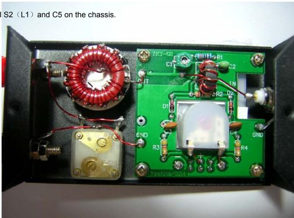
Connect PCB's OUT pad with the S2's 12 foot by using the 24 # enameled wire, and weld GND pad of PCB on the middle foot pad and black terminal of C5 with 24 # enameled insulated wire. Two feet of C5 are welded together and welded to the red terminal.
