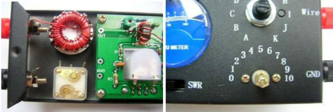
Install S2 (L1) and C5 on the chassis.
