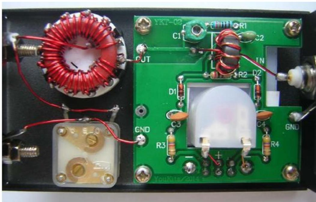
MT1 is designed for the high-impedance long wire antenna, which can be used in the range of 10m to 40m, with the power handling of about 10W ( power handling peak is about 20W), consisting of two parts, namely LC matching circuit and the VSWR power detection circuit .
