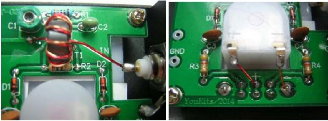
The other end of wire passing through T1 is installed on the pedestal BNC, and pedestal BNC's ground welding piece is soldered on the ground welding piece of PCB. The positive and negative terminals of the meter are connected to the + and - of PCB respectively.
