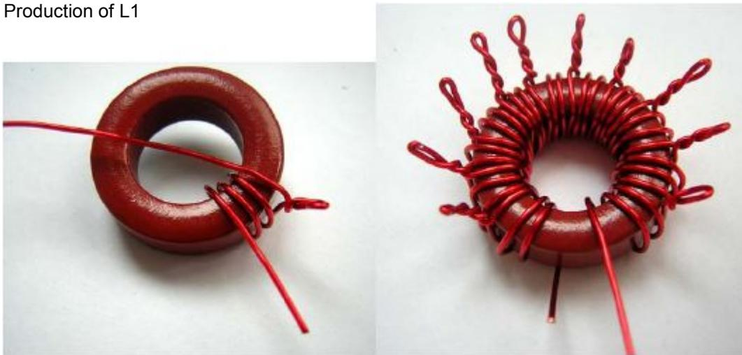
Cut the red 24 #enamel insulated wire about 1m long, and wind on T68-2 magnet ring, then tap for every three loops, totaled 12 taps, with 10 tapped ones and the top the end leads.
