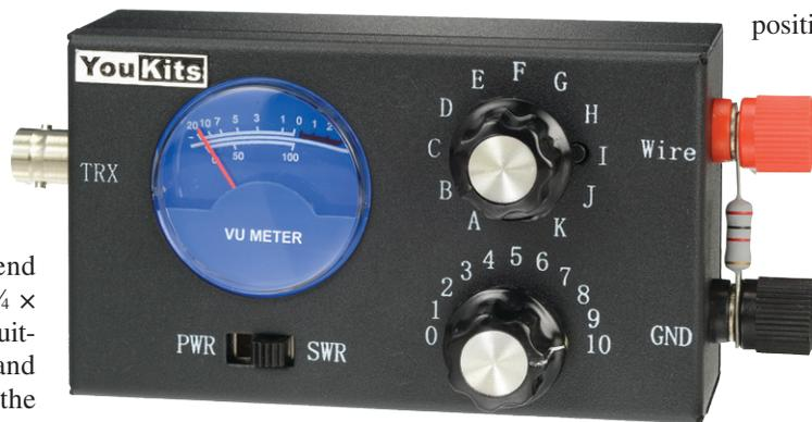
position. If needed, the user can create a table of SWR and power by comparing the MT-1 to a power meter of known accuracy.
