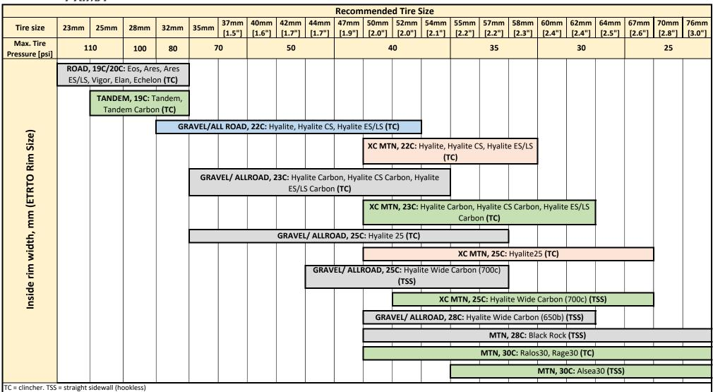
Maximum pressure: If there is a difference between maximum recommended pressure and the tire manufacturer's recommended maximum pressure, use the lower of the two.
