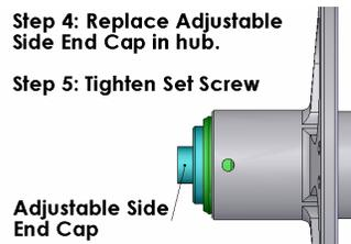
4. Replace the Adjustable-side End Cap carefully, so as not to move the axle or Adjustment Collar.
