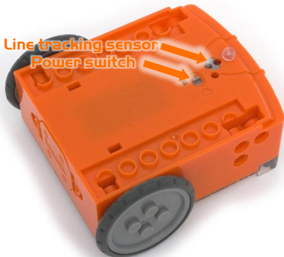
Edison's power switch and line tracking sensor
