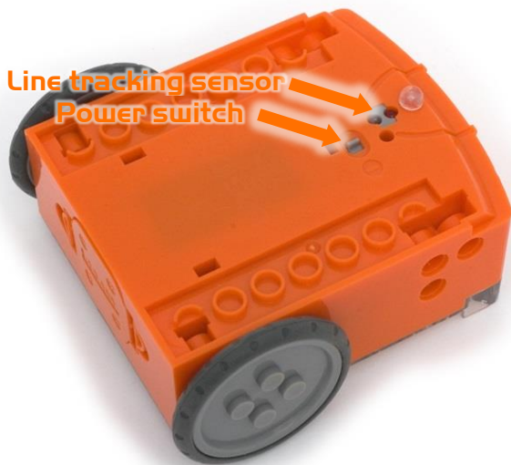
Edison's power switch and line tracking sensor
