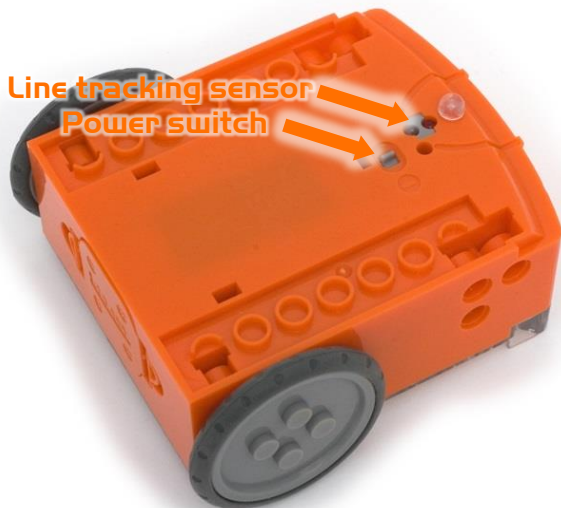
Edison's power switch and line tracking sensor
