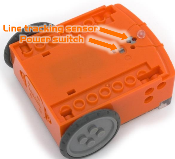
Edison's power switch and line tracking sensor
