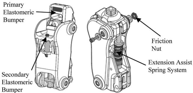
Fig. 2. SASPL knee and components of the swing-phase control system showing frontal-side view (left) and posterior-side view (right).
