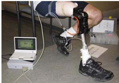
Fig. 4. Testing prosthesis instrumented with potentiometer and accelerometer connected to laptop and data acquisition system
